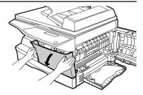
Remove the TD cartridge from the bag. Remove the protective paper. Hold the cartridge on both sides and shake it horizontally four or five times. Hold the tab of the protective cover and pull the tab to your side to remove the cover.
